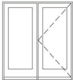
ANDERSEN FRENCHWOOD CENTER HINGED 6-0X6-8 VINYL EXTERIOR WOOD INTERIOR FULL GLASS 7 1/2 JAMB
