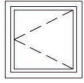
ATRIUM 3-OX3-0 CASEMENT VINYL WINDOW W/ J CHANNEL INSULATED GLASS NO EXTENSION JAMB
