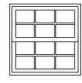
ANDERSEN 3-OX3-0 200 DOUBLE HUNG VINYL WRAP EXTERIOR MATCHING SCREEN WOOD INTERIOR INSULATED GLASS NO EXTENSION JAMB
